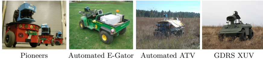
Fig. 1. Some robots that currently use Field D* for global path planning. These range from indoor planar robots (the Pioneers) to outdoor robots able to operate in harsh terrain (the XUV).
